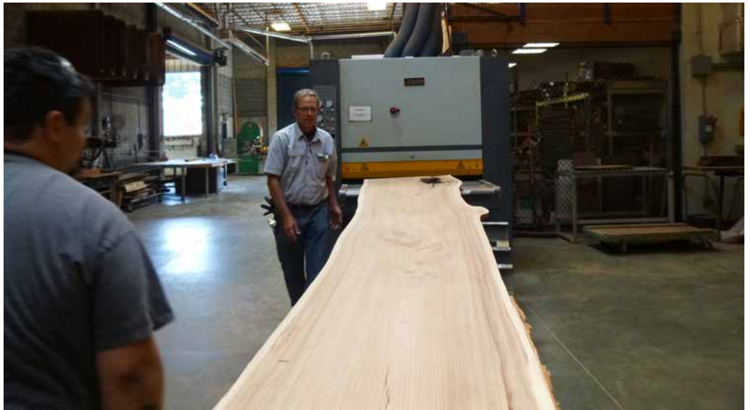
This single piece oak board that will eventually become a bar gets set to go through the sander.
